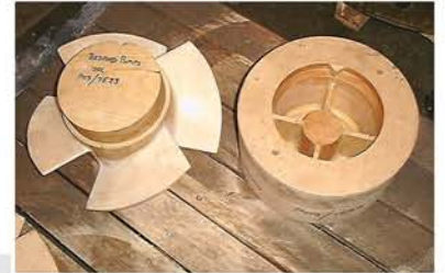
New impeller pattern manufactured by BPL
