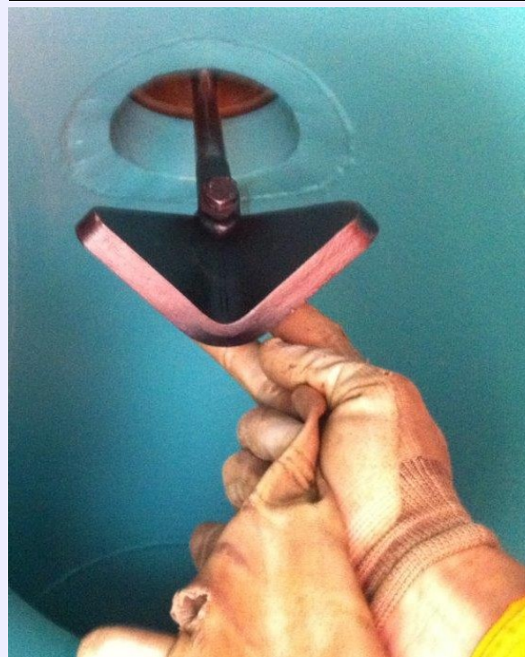
Fish Friendly profiled siphon paddle
