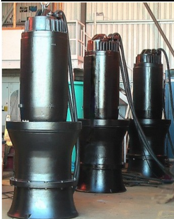
Bedford Pumps SA.80.04.10 pump sets as used at Pinkston
