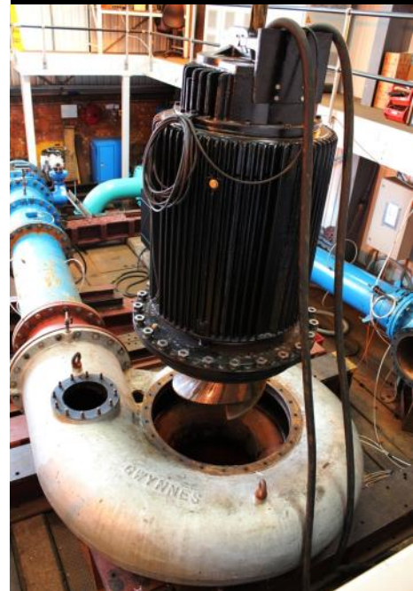
Bedford Pumps new rotating element utilises the existing pump casing
