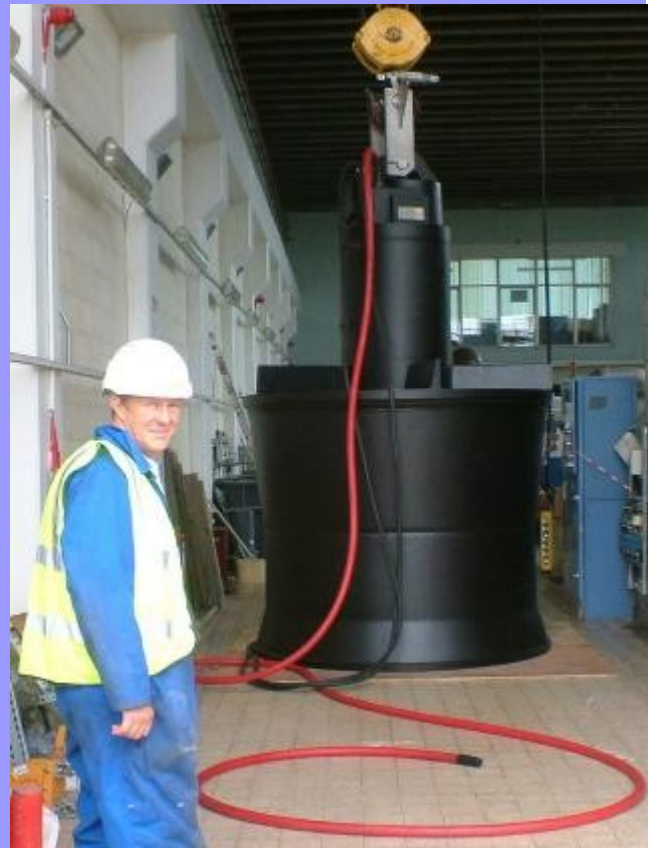
Bedford Pumps' Storm Pump for Altmouth P.S.
